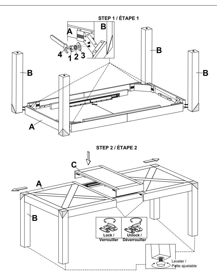
Note: Please use a spirit or digital level and adjust the levelers provided on the legs of your table to ensure the table top it is completely flat. Make sure the top of the legs are aligned to the table top before tightening.
